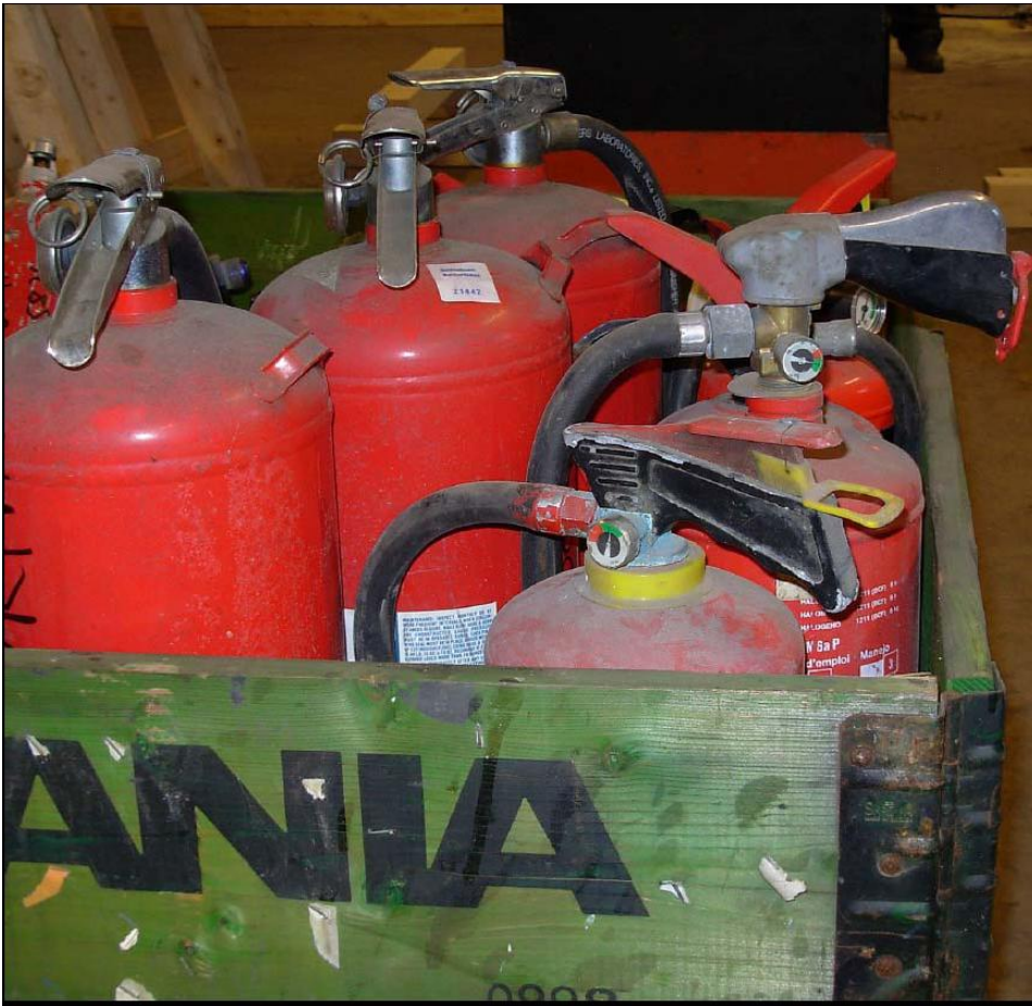
Picture 6. Correct packing of hand-held extinguishers. NOTE: unable to stack on this pallet.
