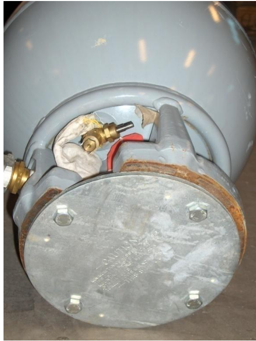
Picture 1. Spherical halon container w/bolted plate.
